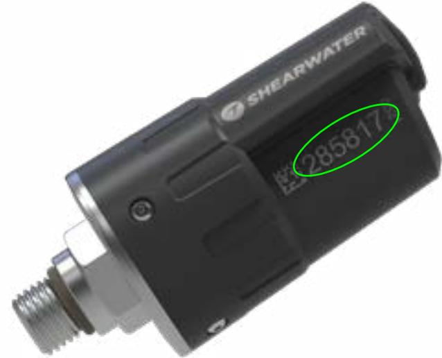
Pair the transmitter by going to the **Tx Setup** menu option, and selecting T1. Turn on T1, then enter the 6-digit transmitter serial number into the **T1 Serial #** setting. You only need to set this once, as it will be permanently saved in the settings memory.
