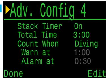
It can be toggled on and off in the Advanced Config. 4 menu. The total time can be set anywhere between and 1h and 9h 59m. The stack timer can be set to count down either when diving, or when the computer is ON. A warning will alert the diver when the stack timer has 1h remaining and an alarm will be displayed when the stack timer has 30 minutes remaining.
