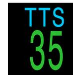
The time-to-surface in minutes. This is the current time to ascend to the surface including the ascent plus all required deco stops.
