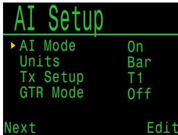
When **AI Mode** is set to **Off**, the AI sub-system is completely powered down and does not consume any power. When on, the AI system increases power consumption by approximately 10%.
