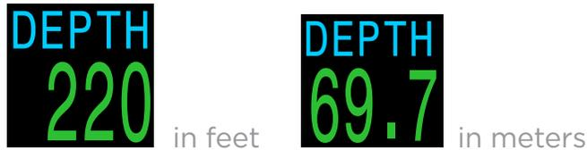
In feet, depth displays with no decimal places. In meters, depth displays with one decimal place up to 99.9m.
