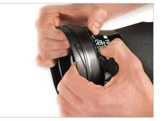
4.4 Press the glove with Spanner Ring evenly into the VIRGO Ring.4.5 Check for creases on the glove as creases may cause leakage.
