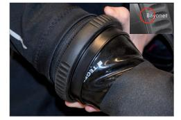
**5.3** When the VIRGO Ring and the VIRGO assembly has been joined together just turn the Lock and Release Ring as the image displays. Turn the Lock and Release Ring until it stops. When this procedure has been made properly you should only be able to see part of the edge of the bayonet (as displayed in the right section of the image box).
