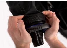
**2.2** Change grip and continue to press the assembly further into the PU-Ring. Work in a 360° pattern so that you don't put uneccesary stress onto the seal and the PU-Ring.
