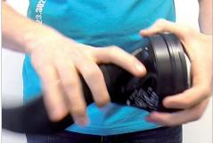
**4.6** Test the strength of attachment by pulling VIRGO Ring and glove in the opposite direction. If the assembly does not hold together, please change the Spanner Ring to a thicker one.
