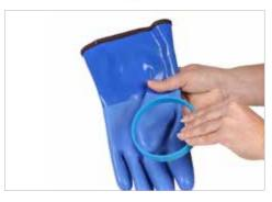
**2.1** Start by finding appropriate Spanner Ring. When pressing the Spanner Ring and glove into the Glove Ring they shall slide without use of excessive force. Use green Spanner Ring for thin fabrics, blue for medium fabrics and yellow for thick fabrics.
