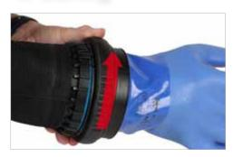
**4.1** Turn the Lock and Release ring in opposite direction compared to the donning procedure. Turn until the Glove Ring and the OBERON Ring are separated. **Tip!** Keep glove on when doffing second ring. The glove provide a higher friction against the rubber ring.
